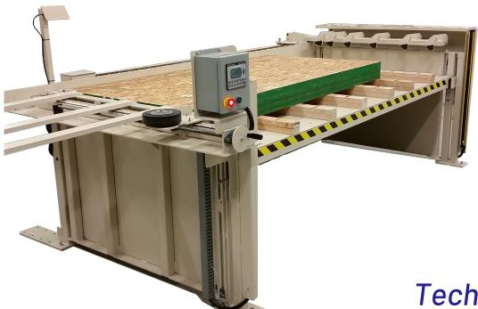
This hydraulic panel feeder is designed to feed glue laminating lines, gang rip-saws, and more. The 8100 serves as an automatic lift, alignment fence, and holdover device in one machine ensuring that your parts are fed consistently every time!
