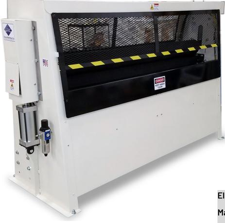
The Evans Machinery Model 0257 Pinch Roller is a key asset for laminating shops, both large and small. The top roller is easily adjustable to the thickness of the work being laminated. Simply insert the provided spacers 1/8", 1/4", and 1/2" to acquire the desired thickness.
