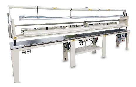
The Evans Midwest Model 0110 Post Former produces counter tops of uniform quality each and every time. It forms most radiuses without time consuming adjustments. The Model 0110 features a pneumatic assisted heater that speeds up your production and cuts down on operator fatigue. This model features an adjustable leaf that allows the operator to easily set the leaf spacing for the build down from 1/2" to 1 1/2".
