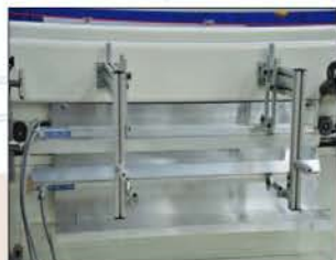
Top & bottom infrared heaters for heating laminate and drying adhesive
