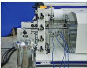
Optional PVA edge spray system for applying adhesive to the edge of core and laminate
