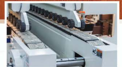
Upper hold-down beam with double row of serrated rollers; transport chain assembly with full-friction carrier blocks
