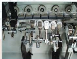
Quick-change forming roller assembly with adjustable, spring-loaded silicone rollers
