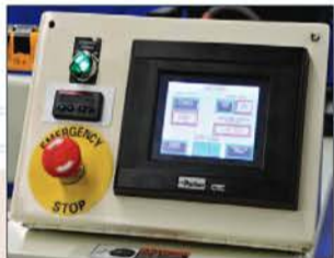
Operator interface with color monitor and PLC controlled sequence of operation
