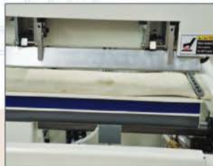
Aluminum cove bar with electronic temperature controls and 90° stops
