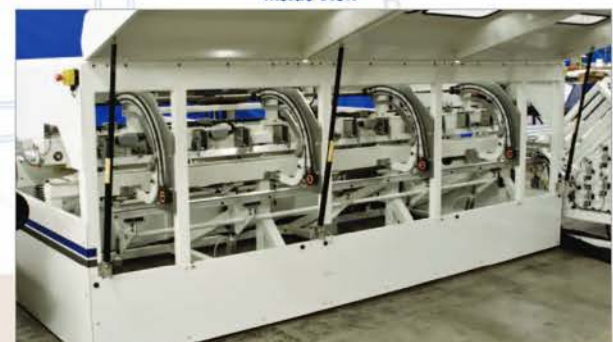
Form bar assembly is electronically driven with chains at four points and includes electronic variable speed control
