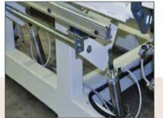
Cove stick placement rack with (5) pneumatic cylinders
